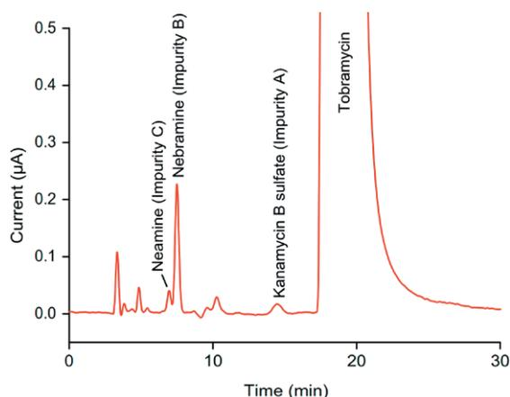
HPLC-ECD chromatogram of Tobramycin antibiotic, composition and impurity analysis according EP monograph. Column: 4.6 mm x 25 cm SDB copolymer. Injection vol.: 20 µL. DECADE Elite equipped with SenCell with Au working electrode and Ag/AgCl reference. Potential: PAD 3 step waveform. ADF 0.5 Hz. Other conditions see Application note 217\_032
