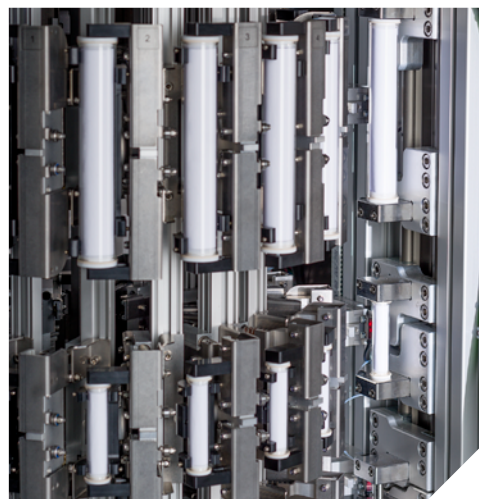
Column carousel is in the rear position with locked columns in the column tower.
