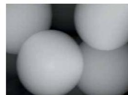
SEM image of 5 µm SweetSep particles
