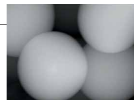
SEM image of 5 µm SweetSep particles
