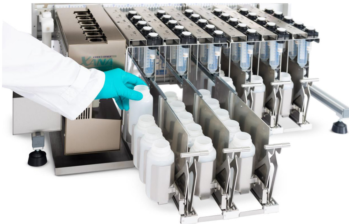
Figure 2. Equipping the bottle rack of the FREESTYLE XANA PFAS TableTop
